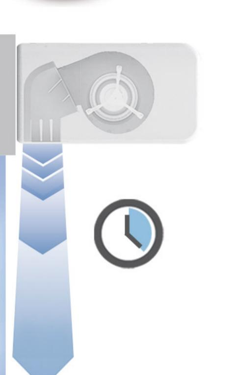
When the door closes, the air curtain remains working at door open conditions for certain time to be ready if it opens again. The power of the unit during this delay time is divided into two strength stages, where the first is stronger than the second one in order to save energy.
